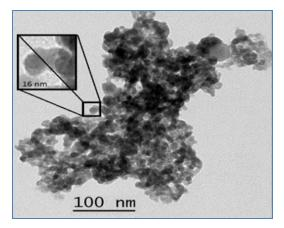
Fig. 4. TEM of gold nanoparticles
