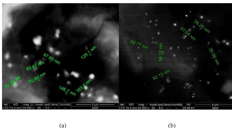
Fig. 5. SEM image (micrograph) of the AgNP structures over the ranges of 70-163nm (a) and 26-91nm (b).
