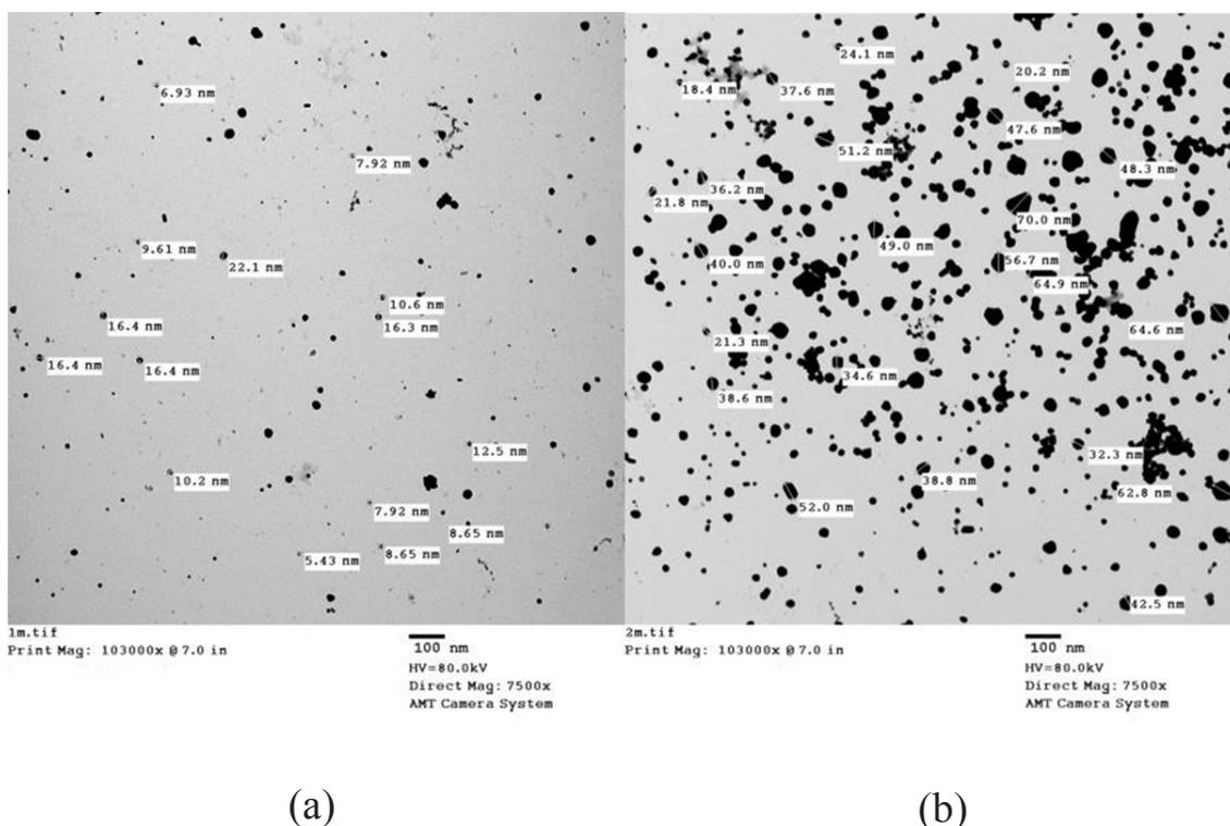
Fig.4. TEM micrographs of AgNPs showing spherical shapes over range 5-22nm (a) and agglomerated structures at 18-70nm (b).
