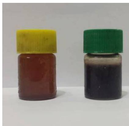
**Fig. 1. Colour intensity, Left: Natural BSH; right: Synthesized AgNPs after 20 min.**
