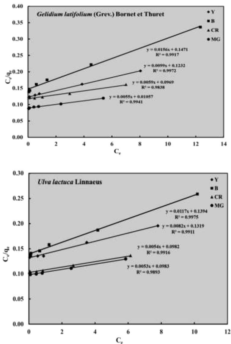
Fig. 2. Linearized Langmuir adsorption isotherms for dyes.
