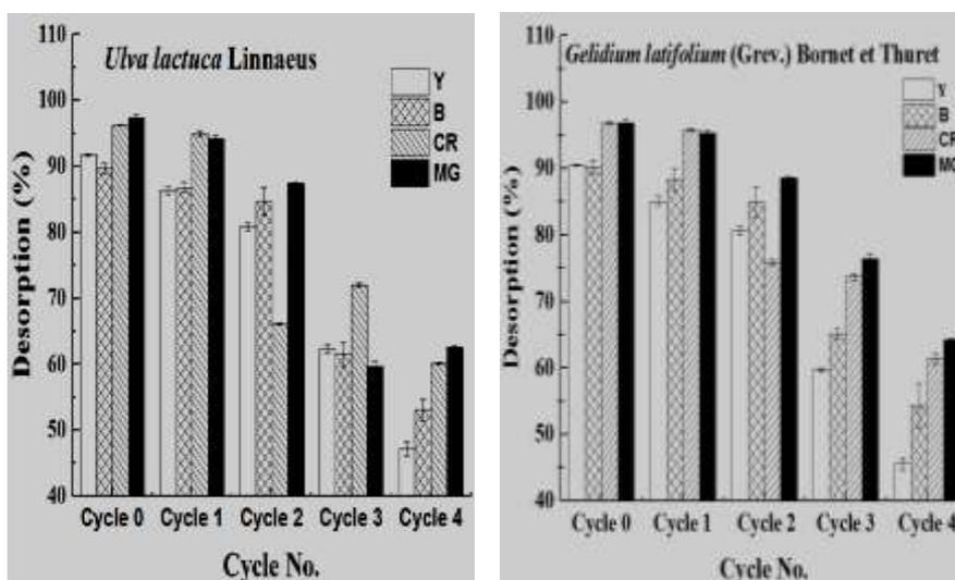
Fig.5. Effect of reuse cycles on desorption efficiency of dyes (Experimental conditions: S/L ratio: 1/500 g/mL, elution time: 4 hours, temperature: 25°C, eluent concentration: 0.01 M, eluent type:  $C_2H_5OH$  for Y and B;  $NH_4OH$  and  $HNO_3$  for CR and MG, respectively).
