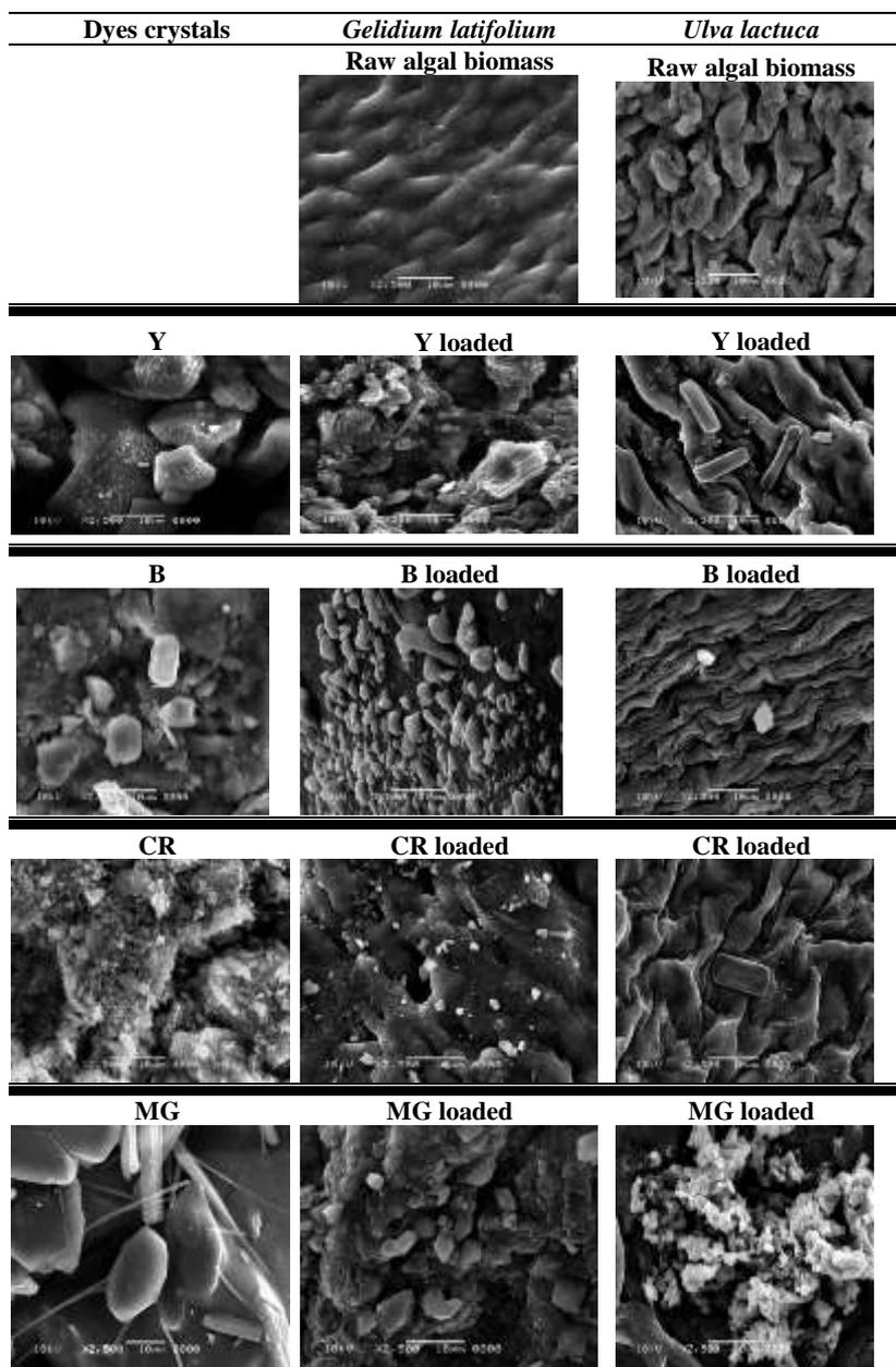
**Fig.7.** The SEM micrographs of dyes crystals and algal biomasses before and after dyes biosorption at X 2500 magnification.
