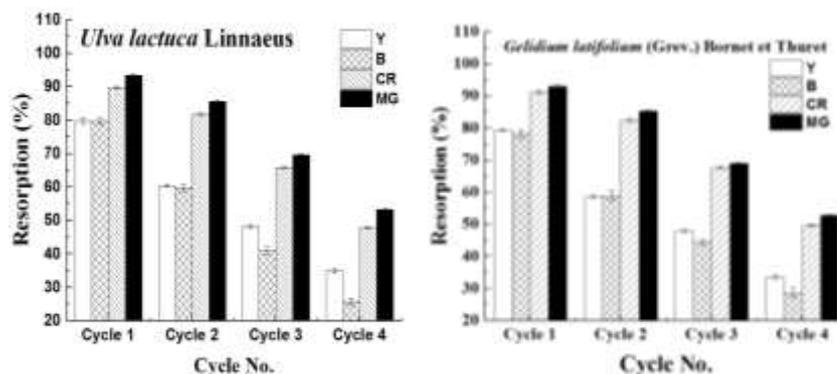
Fig.6. Effect of reuse cycles on resorption efficiency of dyes (Experimental conditions: contact time: 1 hour, temperature: 40°C, initial dye concentration: 400 mg/L, S/L ratio: 1/1000 g/mL, solutions' pH: 1, 2, 8 and 7 for Y, B, CR and MG, respectively).
