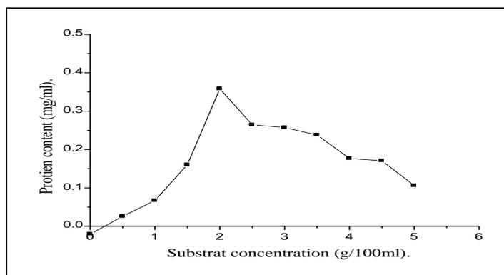
**Fig. 5.** Relation of substrate concentrations to SCP yields produced by *S. cerevisiae* grown on RS1%NaOH at 30°C.
