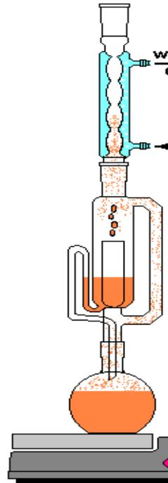
Fig. 2. Soxhlet extractor of marine alga *Dictyota dichotoma*.
