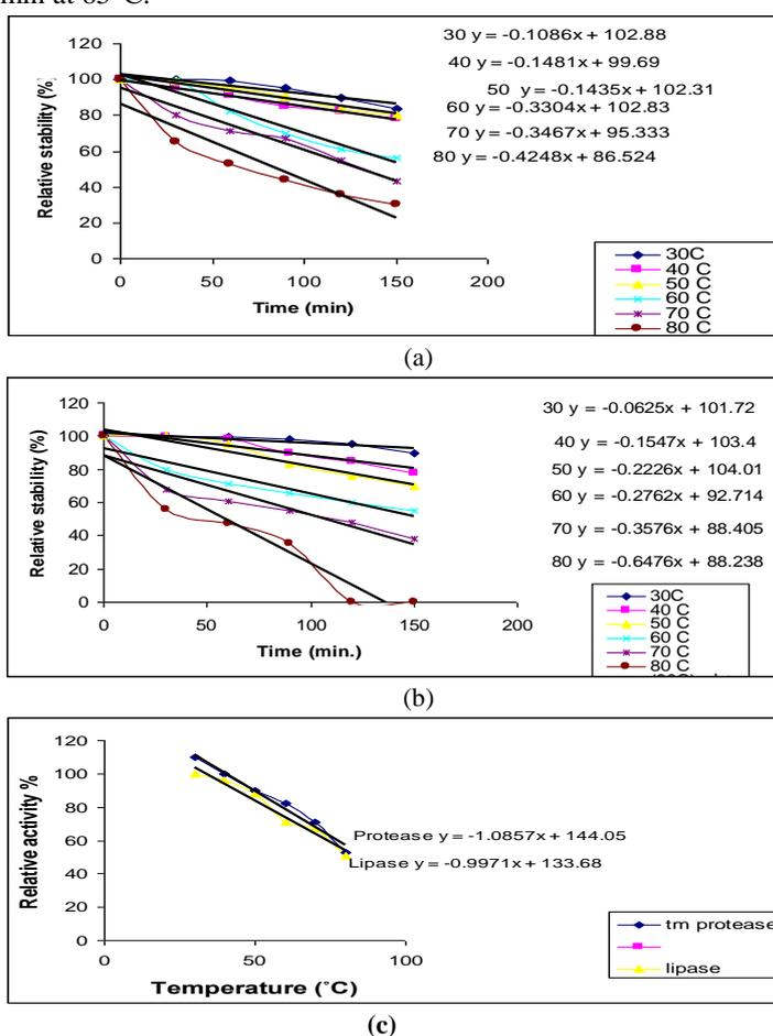
**Fig. 2.** Thermal stability profile of *S. vinaceusdrappus* for both enzymes, after incubation of enzymes at different temperature (30-80°C) and various periods (30-150 min), the residual activity was determined by the standard assay method (a) protease enzyme and (b) lipase; (c) Thermal inactivation profile for protease and lipase,  $T_m$  is temperature degree at which the enzyme retains half of its initial activity at 60 min.
