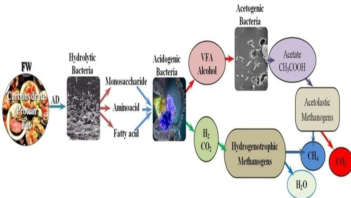
Fig. 2. Stages of anaerobic digestion of food wastes (Srisowmeya et al., 2020).
