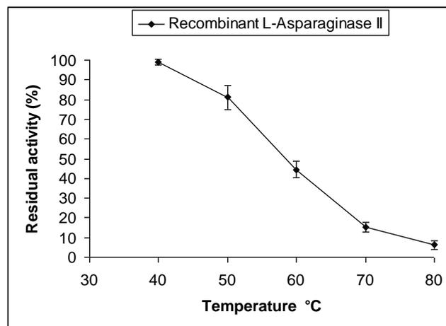
**Fig. 5.** Thermal stability of recombinant L-asparaginase II. Thermal stability was assessed by incubation of recombinant L-ASNase II at 40 to 80°C in 0.05 M phosphate buffer (pH 8.6) for 60 min, and then enzymatic activity was estimated. Residual activity was calculated by comparing the activity to that of the untreated control enzyme, which is taken as 100 %.
