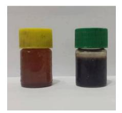
Fig. 1. Colour intensity, Left: Natural BSH; right: Synthesized AgNPs after 20 min.
