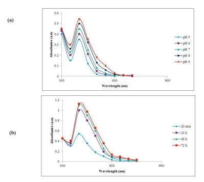
Fig. 2. UV-visible absorption spectra of synthesized AgNPs at different pH values (a) and at different incubation periods for the reaction mixture (b).
