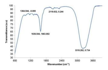
Fig. 3. FTIR spectra of the biosynthesized AgNPs over the wavelength range from 4000-650cm<sup>-1</sup>.
