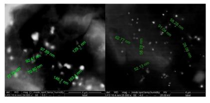
(a) (b) Fig. 5. SEM image (micrograph) of the AgNP structures over the ranges of 70-163nm (a) and 26-91nm (b).
