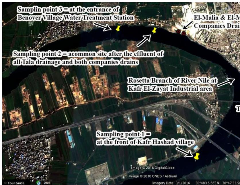
Fig. 2. Representative view for the three points of water sample collection, google earth.
