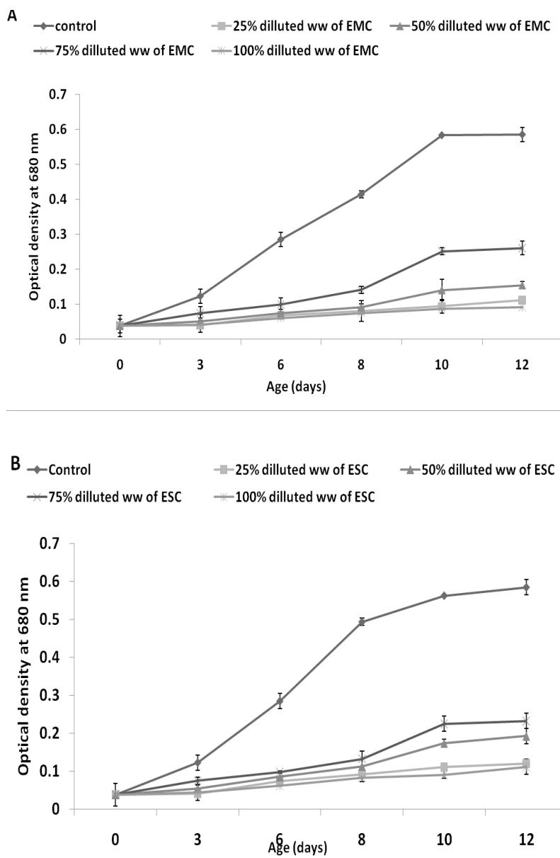
**Fig. 1. Growth curves of *N. oculata* on diluted treated industrial wastewater of (A) El- Malyaa Company (EMC), (B) Salt and soda Company (ESC) with seawater measured as optical density at 680nm. Each point represents the mean value of three replicates; bars indicate standard deviations.**
