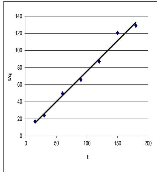
**Fig. 6. Pseudo-second order kinetics of lead adsorption by BLB.**
