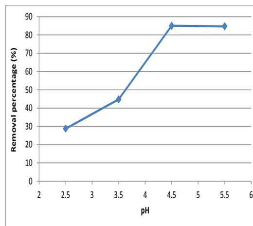
**Fig. 4.** Effect of initial solution pH on Pb(II) removal onto BLB at a lead concentration of 25mg/L, contact time 90min and biomass loading weights 8g/L.
