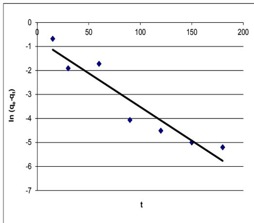
**Fig. 5. Pseudo-first order kinetics of lead adsorption by BLB.**
