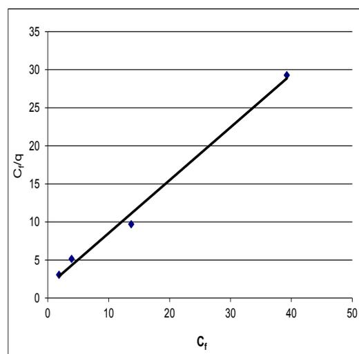
Fig. 9. Langmuir plot of lead adsorption by BLB.
