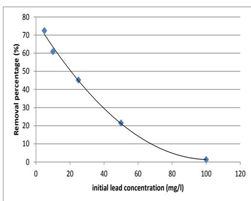
Fig. 8. Effect of lead initial concentration on its removal by BLB at contact time 90min, initial solution pH 4.5 and biomass loading weights 8g/L.
