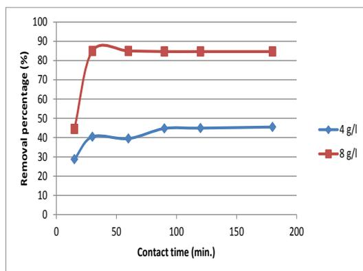
**Fig. 3.** Effect of contact time on Pb(II) removal onto BLB at a lead concentration of 25mg/L, solution pH 4.5 and biomass loading weights (4 and 8g/L).
